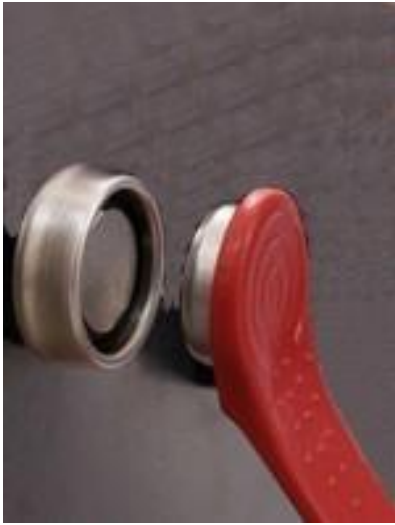
Fob reader on each courtside controller.
